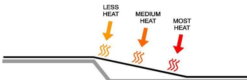
Heat the vinyl to soften and re-tension the film over the bridged area, ensuring heat is then concentrated to the vinyl opposite the recess (this ensures the stretch comes from this area not the recessed area)
