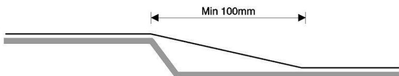
For application of film into single step shallow recesses 3M 1080cv3 series should be bridged as normal, leaving a minimum of 100mm of film bridged, this may increase depending on depth of recess.
