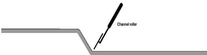
Once the vinyl is in place and still warm (35-40°C), the small channel roller must be used in the recess. This is to ensure maximum bond in the recess. The channel roller applies a large amount of pressure to a small surface area, which is a lot more effective than your finger or the thin edge of a squeegee.
