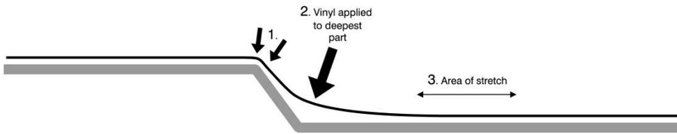
Vinyl is to be applied to the deepest part first with stretch coming from the flat, non-recessed area. Any trapped air on flat areas can be worked out progressively with the aid of Comply™ air release technology.
