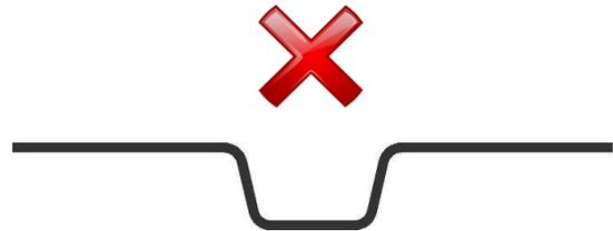
B) 3M 1080cv3 series is not suitable for U shaped recesses, or complex curves. 3M IJ380-10 is the only vinyl suitable for these applications. (3M IJ380-10 application bulletin also available)
