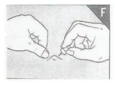
With the COVER STYL'® film, it is not necessary to drill the bubbles so that the air escapes. Cut the film excess with a cutter and a straight rule.
