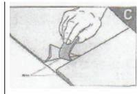
Remove the film and the release liner
