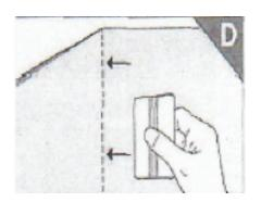
Mark the wedge angle along the length of the panel with the squeegee.
